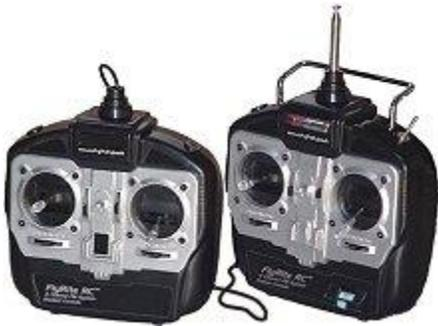
In conventional BB systems the transmitters are joined together by a cable; the instructor holds the master transmitter while you, the student, hold the slave transmitter. With the flick of a switch the instructor can hand over or take away complete control from you, without having to take the transmitter from your hands.
